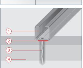
Locate the next mounting rail (1) to the right of it with a gap of 30 mm.
