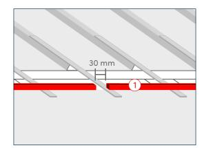
The mounting aids are cut to size by the solar installer, e. g. from a piece of wood.
